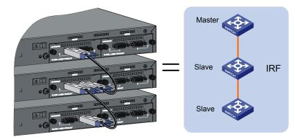
Figure 3-26 The ring connection mode
